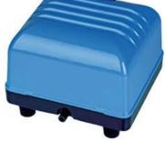
Model V-20 Power:15W Voltage: 230v Pressure: >0.02Mpa Output:20 l/min Noise: <40dB Weight: 2.5 kg Size: 230x185x180mm
